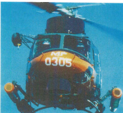
■ Variants of the A244/S torpedo have been sold to more than 15 navies. Here the weapon is being carried by an AB 212 helicopter.
