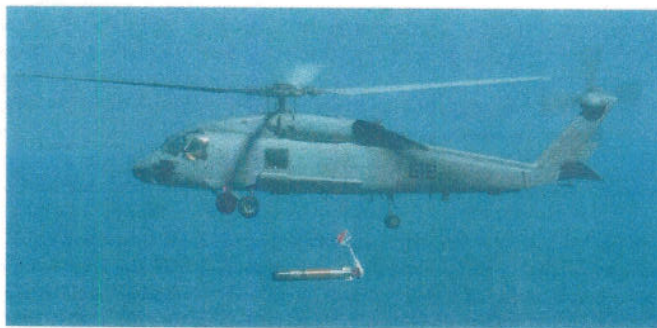
A Mk 54 lightweight torpedo being launched from a US Navy SH-60F helicopter.
